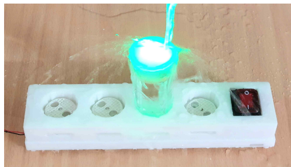
■ Water inflow scene during power connecting
